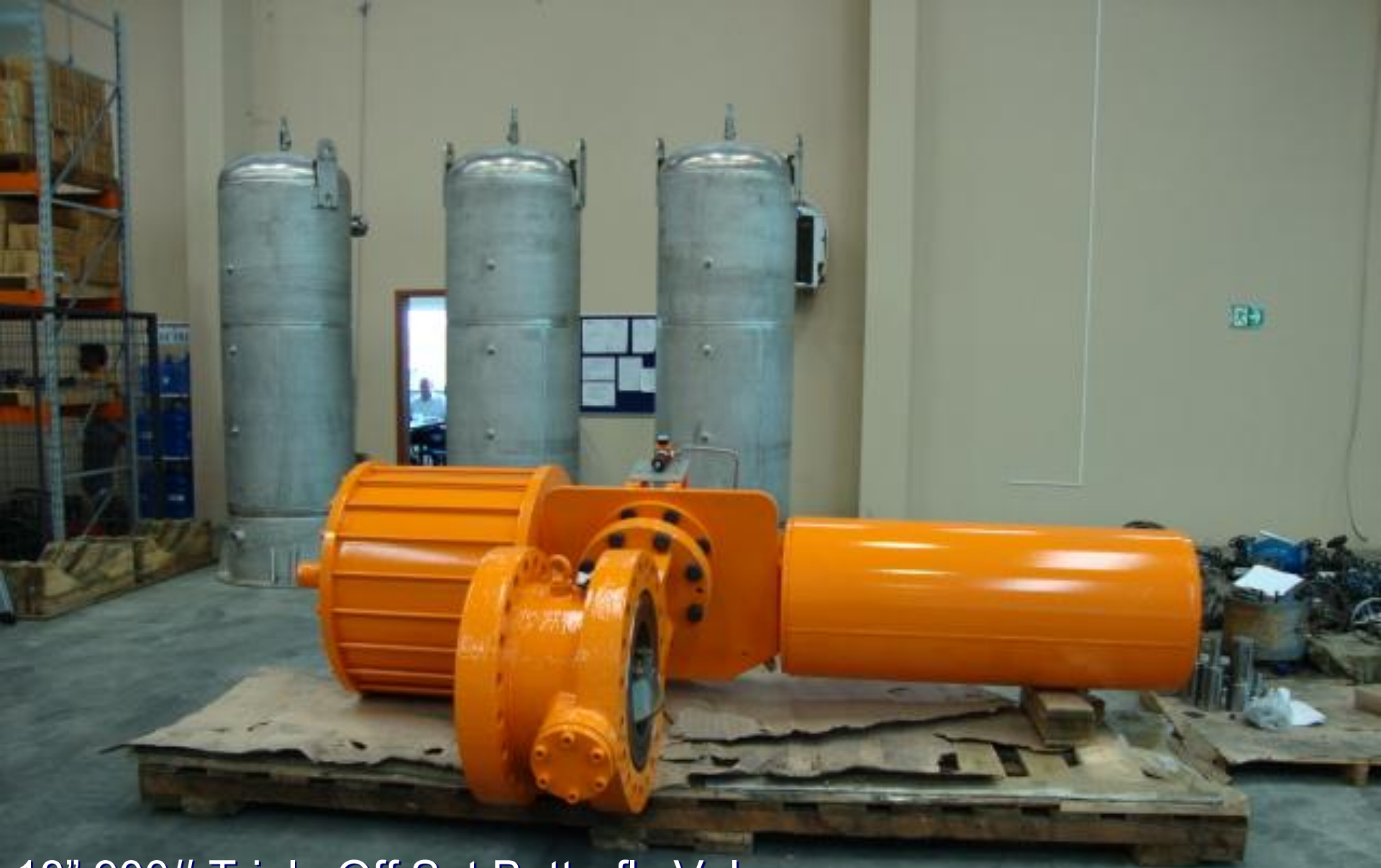
18" 900# Triple Off Set Butterfly Valve with emergency air supply tank + pneumatic actuator and accessories
